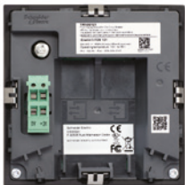
Connection with FDM121 display unit.
