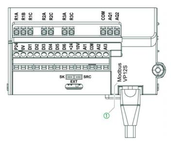
① Modbus VP12S: This is the standard Modbus serial link marking. VP•S means connector with power supply, where 12 stands for the 12 Vdc supply voltage.
